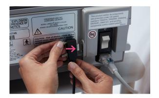
**3. Turn** both thumb screws clockwise until finger tight
