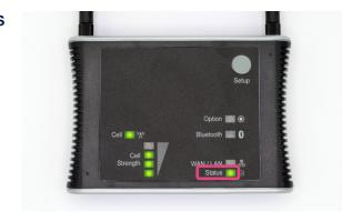
5. Observe the Cell Strength lights while slowly rotating the antennas on the back of the Gateway. Position them for the strengest cell strength
